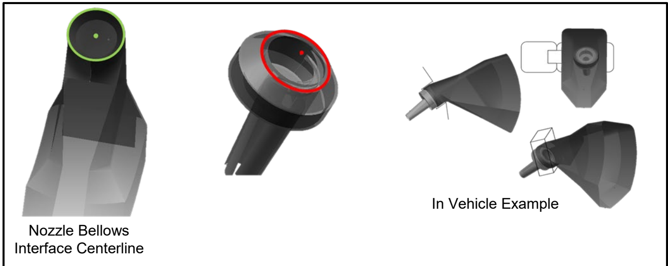
Figure 4F Zone Placement for Vehicle Usage for Comparison to Nozzles with Spout Angles Outside of the Range Specified in Table 4-2 ( S_{\alpha} of 19.5° to 26.0°)
