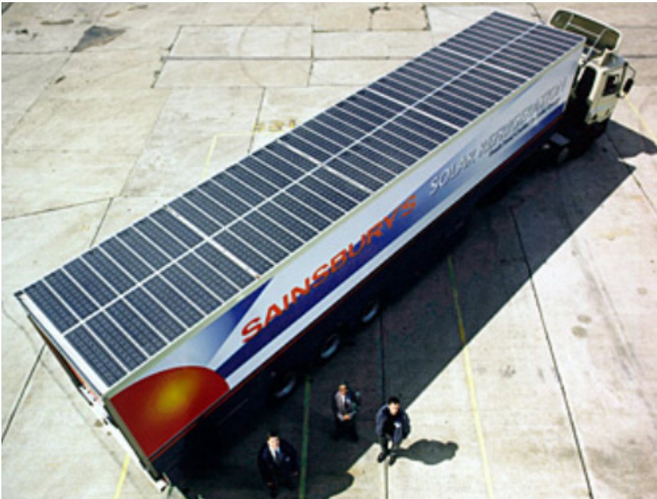
Figure 31: Trailer with Solar Assist 184
