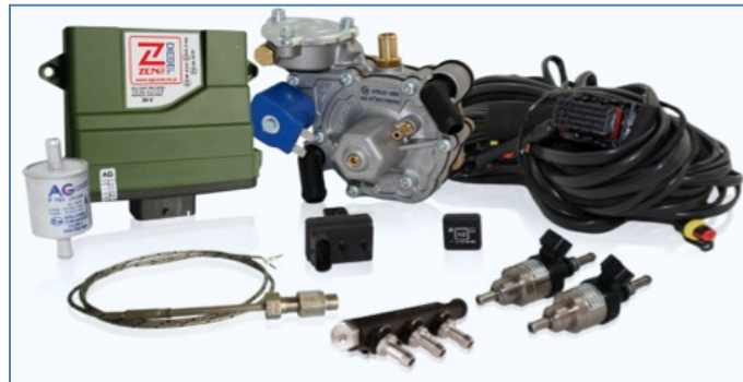
Figure III.F-5: Diesel to CNG Conversion Kit (CNG United™)
