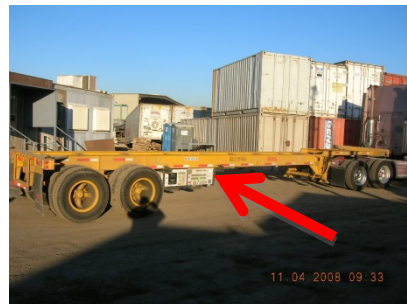
Figure ES-5: Under-slung TRU Genset
