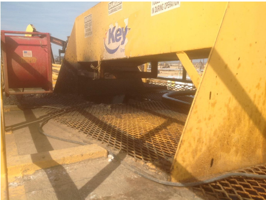
Figure 2-2 Collection Box on SandX Recirculation Tank
