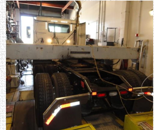
ARB Heavy-Duty Chassis-Dynamometer set-up
