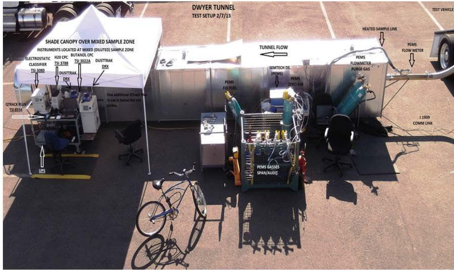
Figure II-7 – Total view of the testing experiment for a Parked Regeneration at Depot Park
