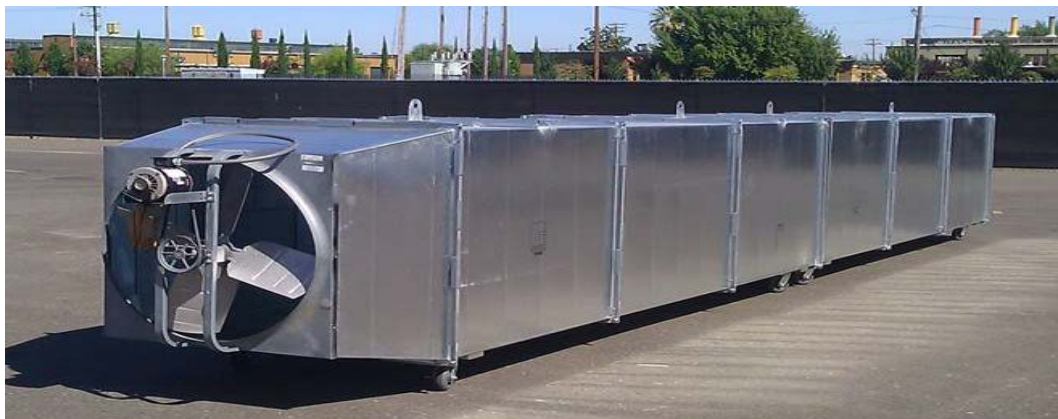
Figure ES-1 Small wind tunnel designed for parked and active regenerations
