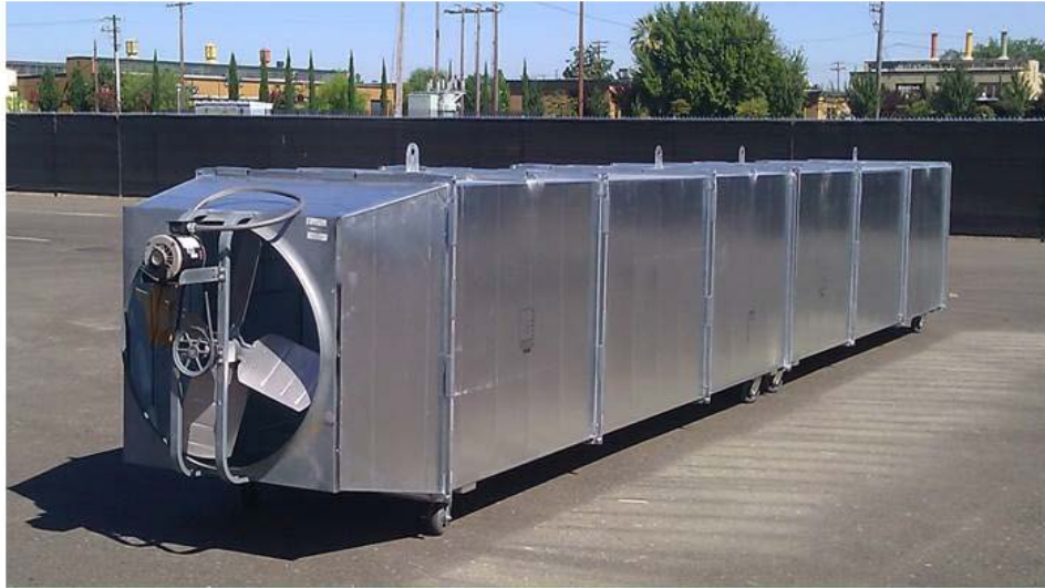
Figure II-1 – Small wind tunnel with attached whole house fan. Tunnel length is 30' and the cross-sectional area is 4' by 4'.
