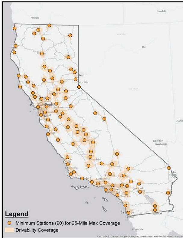
FIGURE 55: GEOGRAPHICALLY OPTIMIZED STATION NETWORKS TO MINIMIZE THE NUMBER OF STATIONS NECESSARY TO PROVIDE COVERAGE TO CITY CENTERS SUBJECT TO AN X-MILE LIMIT OF COVERAGE
