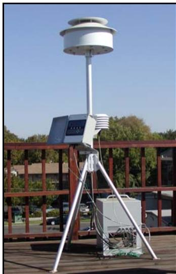
We chose the Beta Attenuation Monitor (BAM) for use in California and have installed monitors at 101 sites. Recently, the U.S. Environmental Protection Agency (U.S. EPA) designated certain models of the continuous monitors as Federal Equivalent Monitors (FEM). They are considered to provide equivalent data to the Federal Reference Monitors and can therefore be used to determine compliance with federal standards. California has deployed 47 of these FEM monitors.
