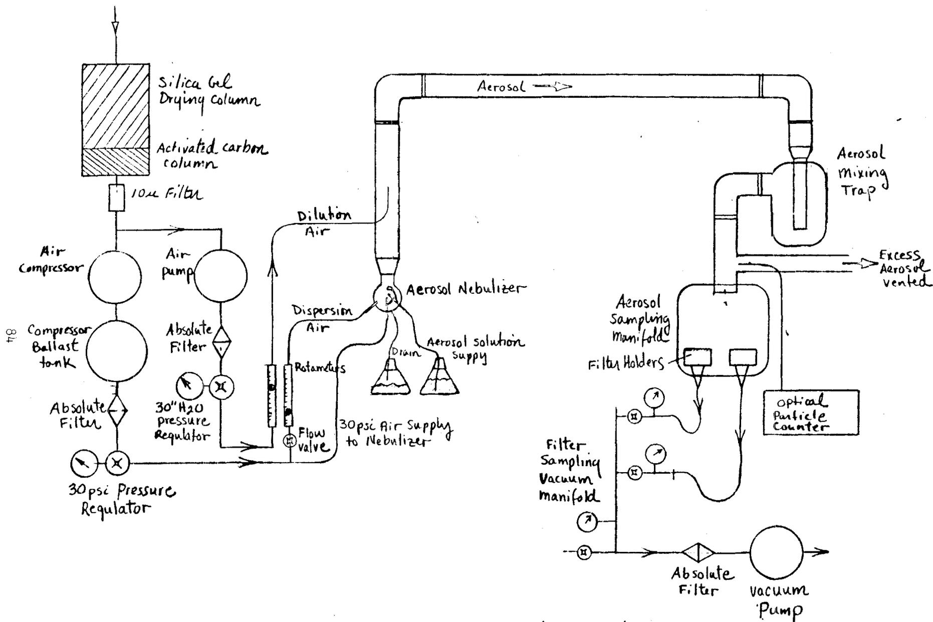
Ammonium Sulfate Salts Aerosol Generator
