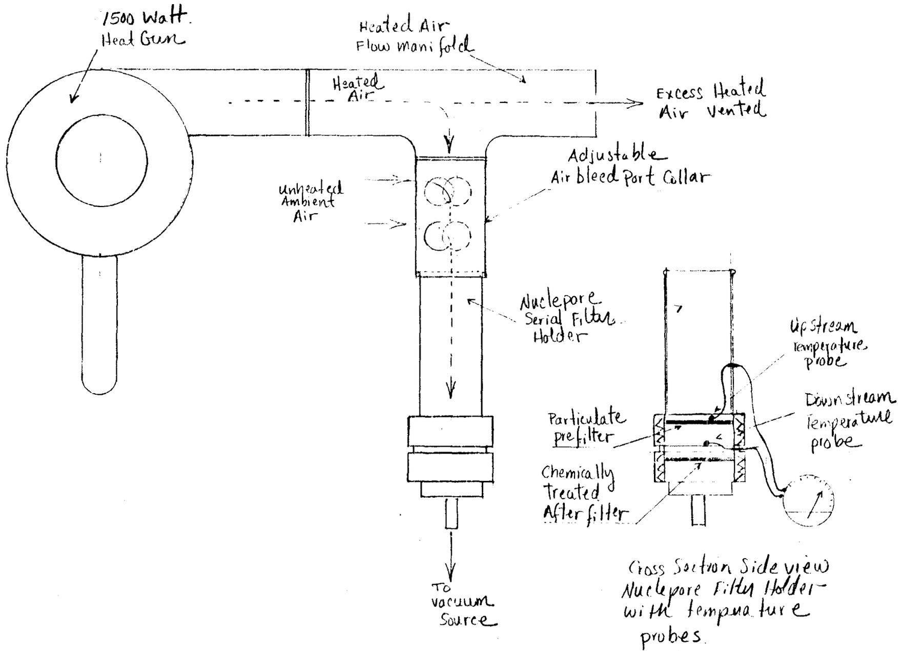
Figure F-1 System for Heating Filter Sampler to Desorb  $\text{NH}_3$  and  $\text{HNO}_3$
