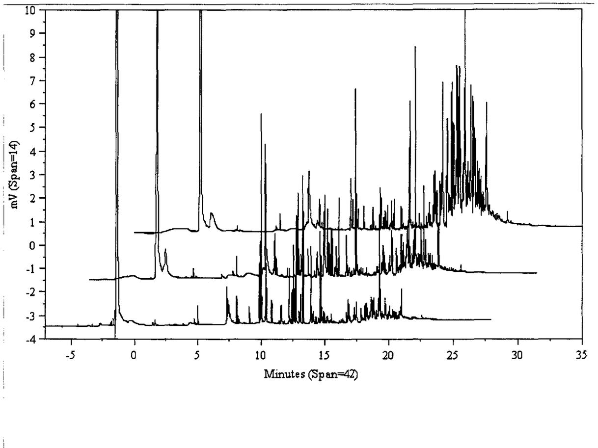
Figure 5-3. Lower chromatogram: canister sample from 0.5 mile from Pico Rivera Station; middle chromatogram: typical “ambient” air sample at Pico; top chromatogram: room air in the Pico Station. The first large peak is CO<sub>2</sub>. Each chromatogram is offset with respect to the abscissa so that the beginning of each trace is at 0.0 minutes.
