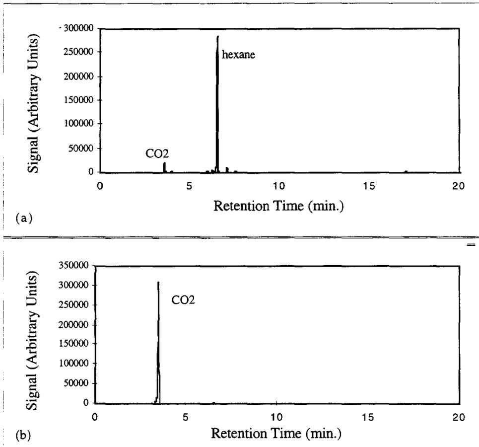
Figure 2-5. Hexane standard (20.2 ppm, 100 mL @ 50 mL/min trap I temp. = -70 °C), (a) without oxidation catalyst; (b) with oxidation catalyst.
