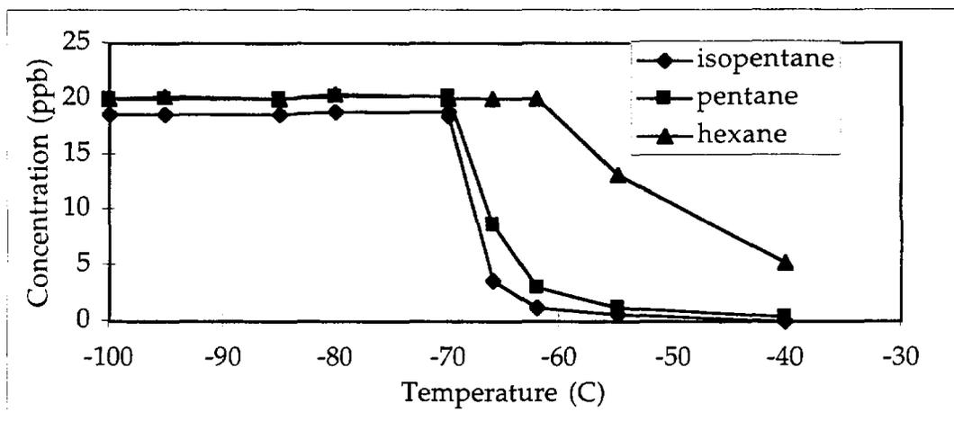
Figure 5-2. Trapping efficiency as a function of trap temperature for isopentane, pentane and hexane. Sample flow rate was 50 mL/min.
