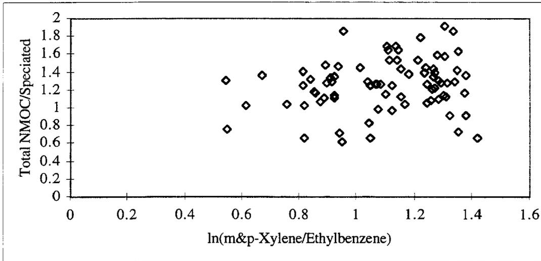
Figure 5-10: Ratio of Total NMOC/Speciated is plotted versus the  $\ln$  (m&p-xylene/ethylbenzene).
