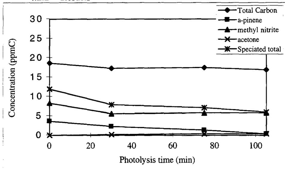
Figure 4-1. Concentrations of TNMOC,  $\alpha$ -pinene, methyl nitrite and acetone as a function of photolysis time (the sum of the time the UV lights had been on), for experiment 1.
