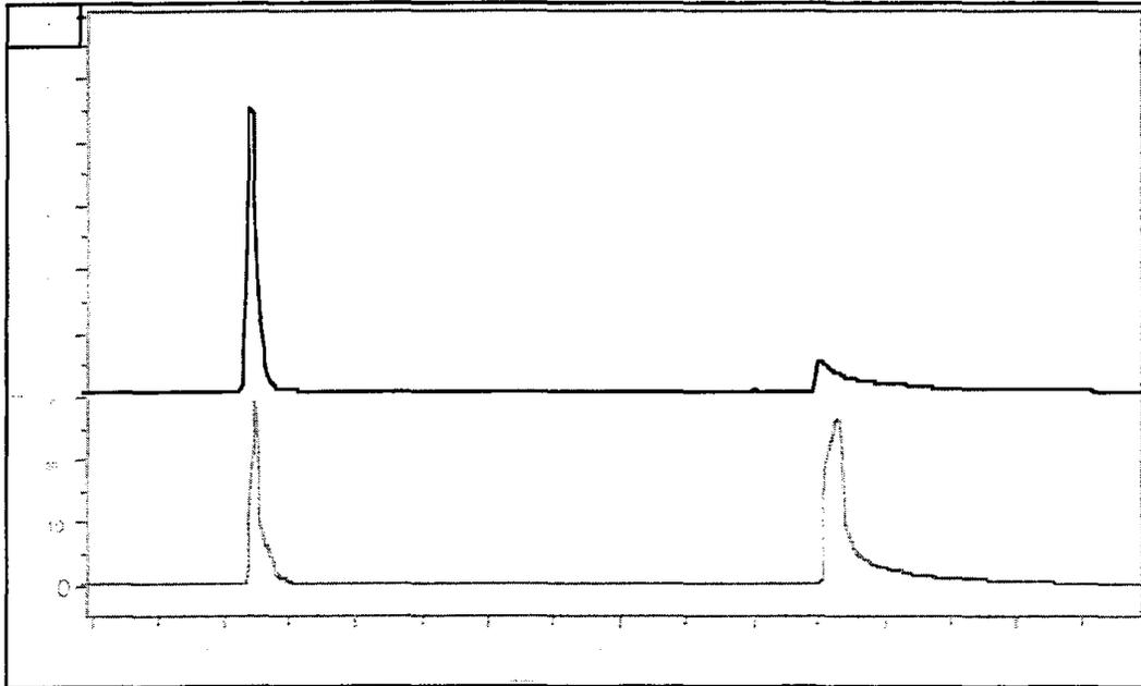
Figure 4-4. Speciated chromatograms of methyl nitrite with heated sample line (lower chromatogram) and without heated sample line (upper chromatogram).
