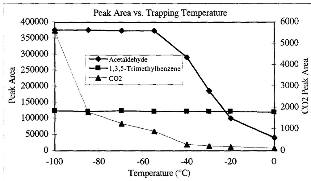
Figure 2-2. Trapping vs. temperature of acetaldehyde and 1,3,5-trimethylbenzene. This mixture was made in ultra high purity nitrogen, thus the CO<sub>2</sub> peak is very small. The acetaldehyde and 1,3,5-trimethylbenzene concentrations are about 12 ppm, and 0.6 ppm respectively.
