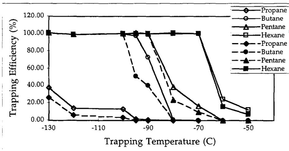
Figure 2-7. Trapping of several alkanes as a function of temperature in the parallel inlet. Column 1 (open symbols, solid lines) is normally the TNMOC channel; for these tests the sample was not oxidized. Column 2 (solid symbols, dashed lines) is the Speciated VOC's channel.
