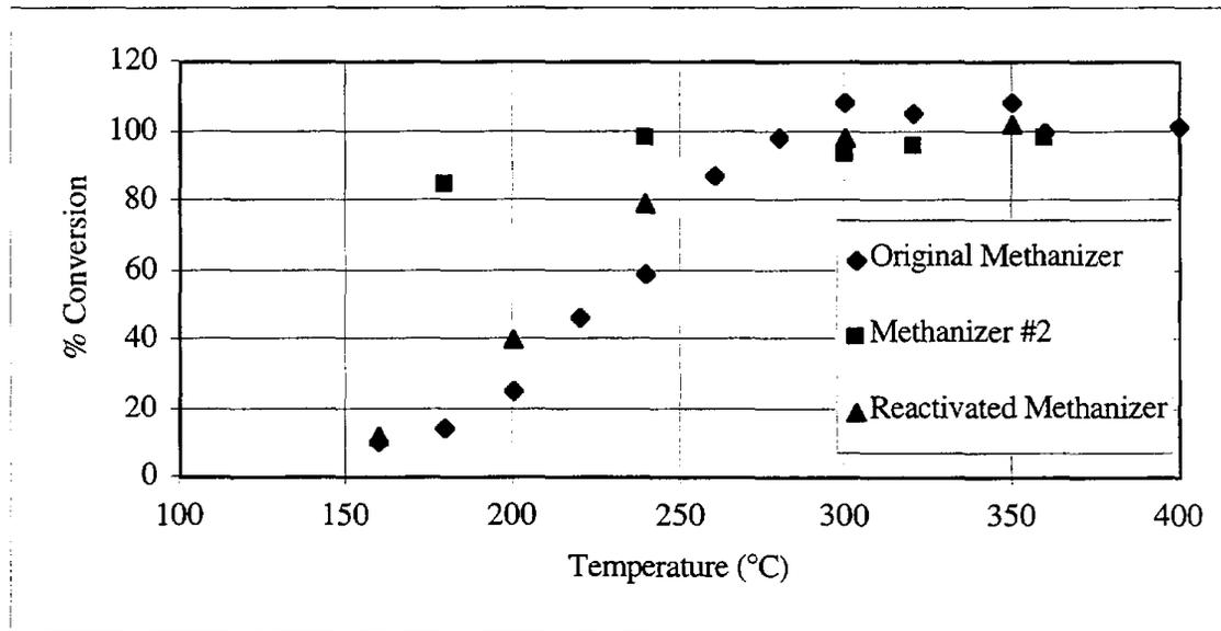
**Figure 2-6. The Temperature Dependence of The Methanizer Catalyst Tested with a n-hexane Standard at 1.08 ppm**
