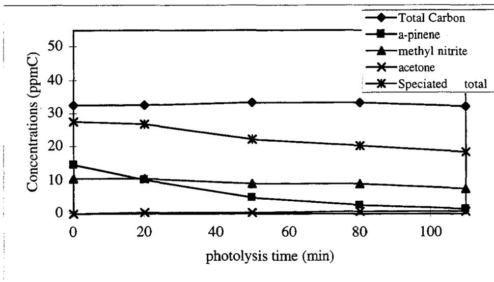
Figure 4-2. Concentrations of TNMOC,  $\alpha$ -pinene, methyl nitrite and acetone as a function of photolysis time (the sum of the time the UV lights had been on), for experiment 2.
