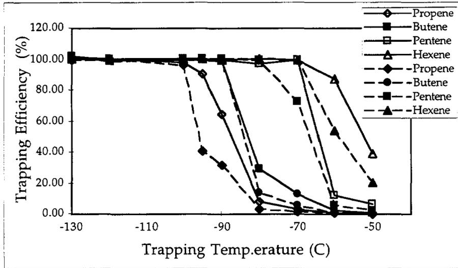
Figure 2-8. Trapping of several alkenes as a function of temperature in the parallel inlet. Column 1 (open symbols, solid lines) is normally the TNMOC channel; for these tests the sample was not oxidized. Column 2 (solid symbols, dashed lines) is the Speciated VOC's channel.
