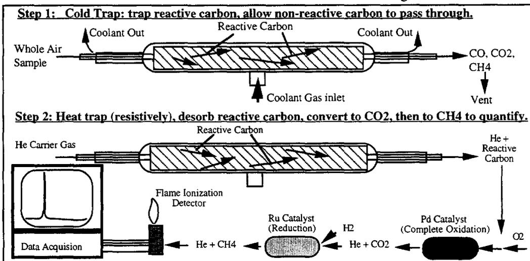
Figure 1-1. Process schematic of the approach for the total TNMOC measurement.
