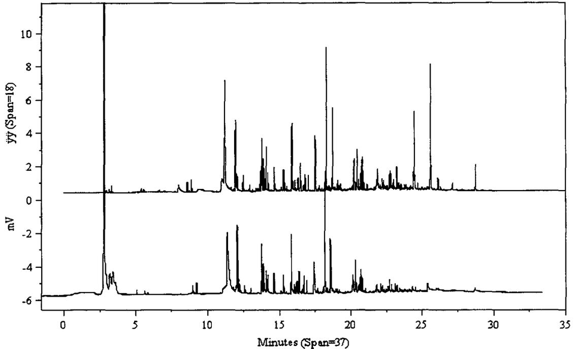
Figure 2-3: Chromatograms from the canister sample analyzed “speciated column 1” with methanizer (lower chromatogram) and “speciated column 2” (upper chromatogram). The large peak at 3.5 minutes is CO<sub>2</sub>, and this is only visible on Column 1 which uses a methanizer. The heaviest peaks that elute after about 22 minutes appear to be lost in the methanizer (lower chromatogram). These chromatograms are not offset with respect to the abscissa.
