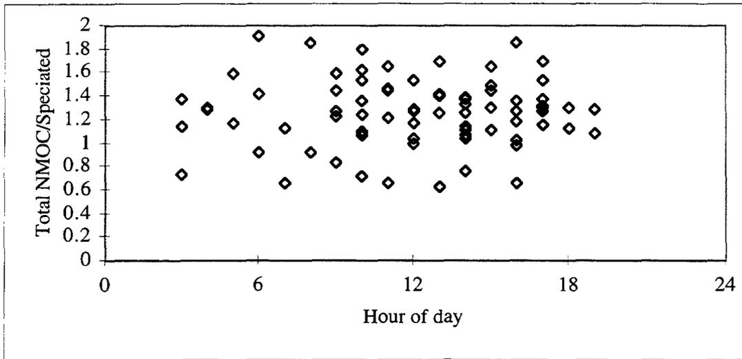
Figure 5-6: Ratio of Total NMOC/Speciated VOC's (T/S) over the course of a day for 83 pairs of measurements taken between September 4 and October 10.
