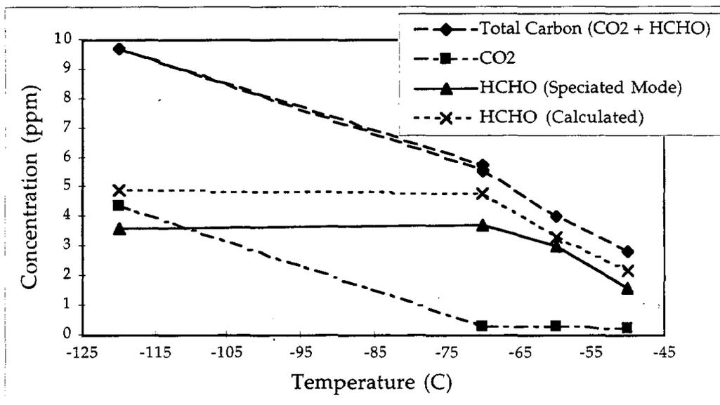
Figure 2-1: Concentration of CO<sub>2</sub>, HCHO and Total Carbon as a function of the temperature of trap 1. The actual amount of HCHO was calculated as the difference of the Total NMOC and the amount of CO<sub>2</sub> trapped.
