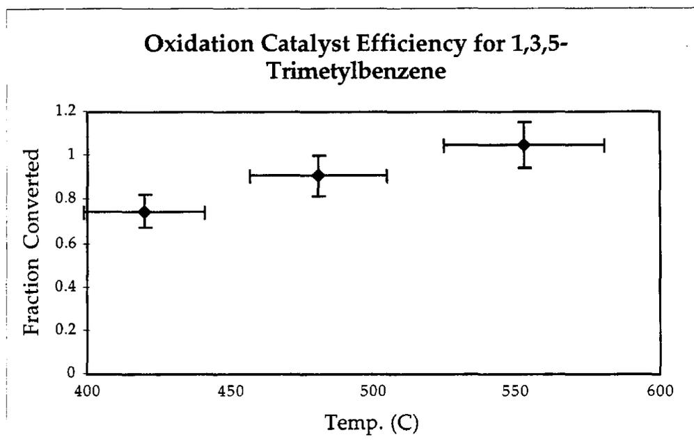
Figure 2-4. Oxidation Catalyst Efficiency for 1,3,5-Trimethyl benzene
