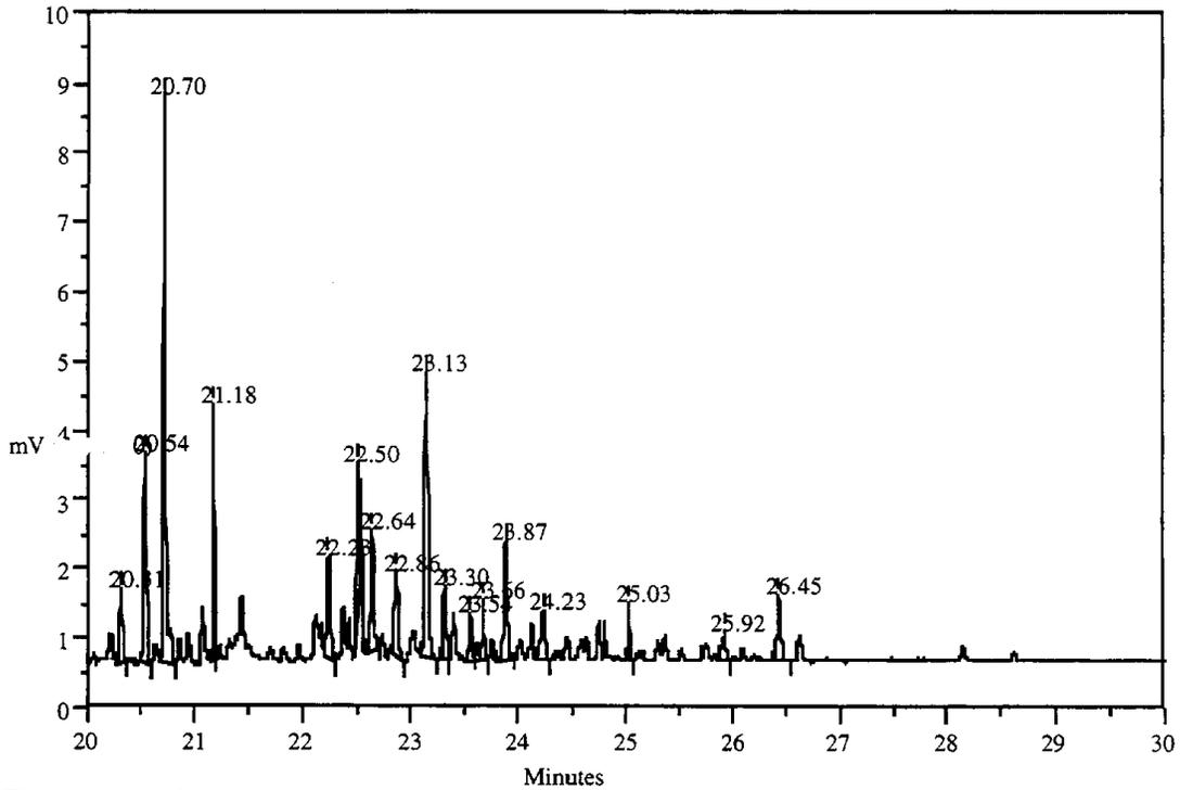
Figures 5-4: Chromatograms from the Speciated VOC's of an ambient air sample taken on 9/9/1997 at the Azusa site from 11:00 to 11:40
