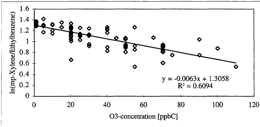
Figure 5-9: ln(m&p-xylene / ethylbenzene) versus the O<sub>3</sub> concentration.
