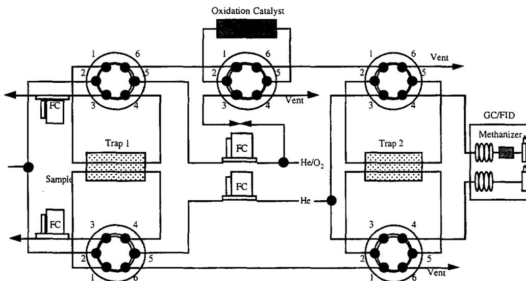
Figure 1-2. Flow schematic for the Reactive Carbon Analyzer. FC = flow controller.
