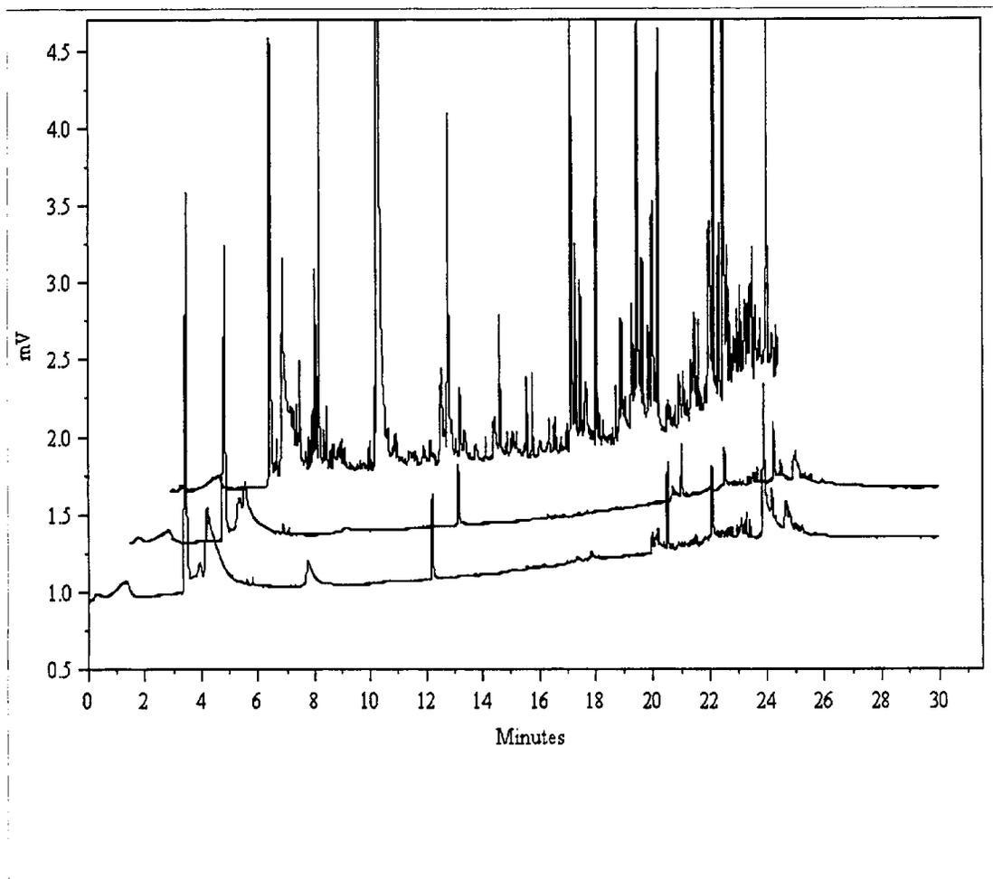
Figure 5-1. Chromatograms showing the effect of sample line choice. All runs used a 100 mL sample of vapor from a liquid nitrogen tank. Upper chromatogram: heated Teflon line, no by-pass flow, middle chromatogram: heated Teflon line, with bypass flow, and lower chromatogram, unheated Teflon line, no by-pass flow. Each chromatogram is offset so that the beginning of each trace is at 0.0 minutes.
