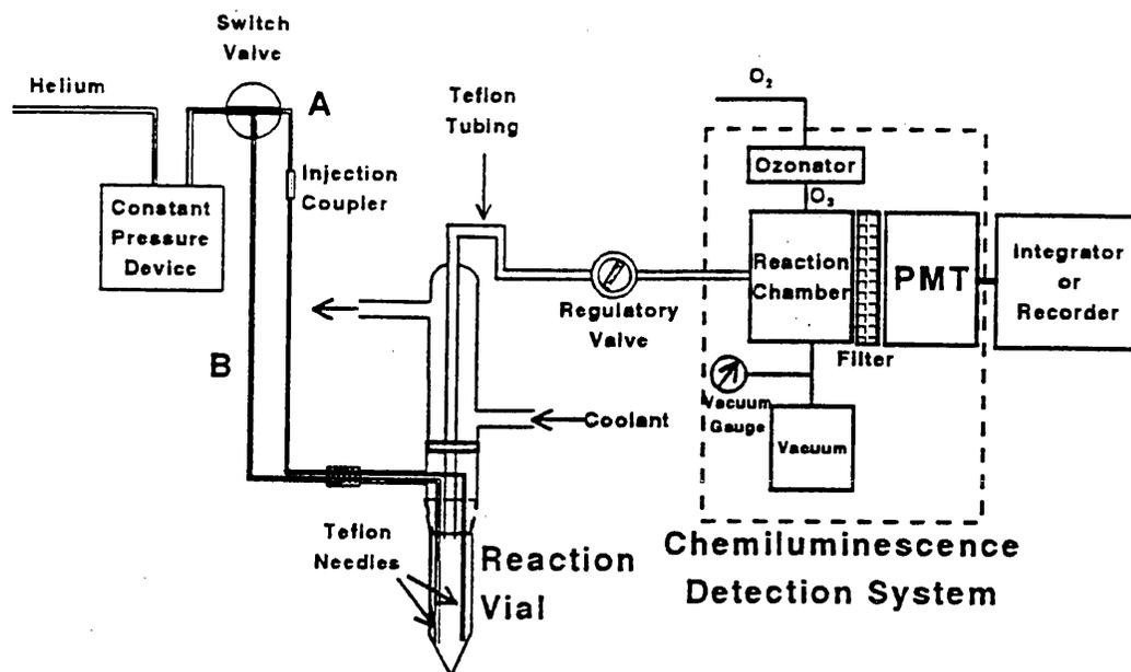
Figure 4. Schematic of the denitrosation analysis system.
