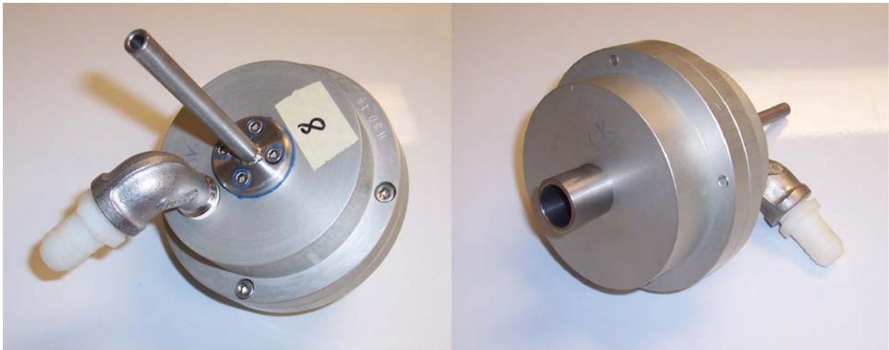
Figure 4. Photo of the virtual impactor. Its cut point is 2.3 micron.
