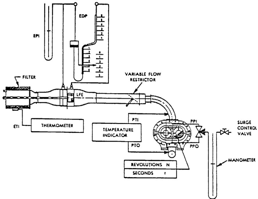
FIGURE F78-5--PDP-CVS Calibration Configuration.
