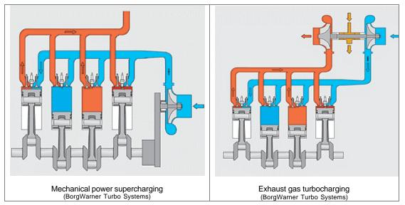
Figure 5-2: Schematics for Supercharged and Turbocharged Engines
