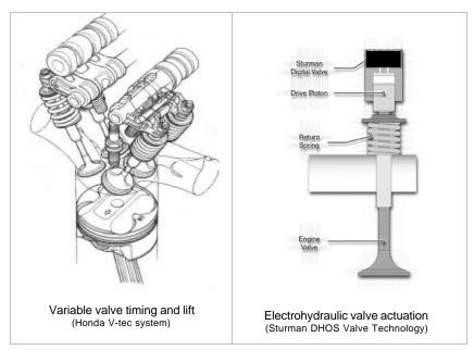
Figure 5-1: Two Variable Valve Systems
