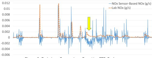
Figure 3. Emissions Comparison Over Hot FTP Cycle
