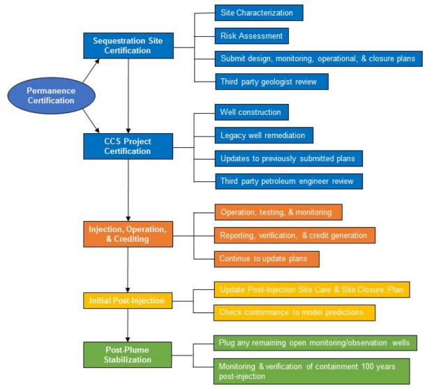
**Figure 3.** Application process flow diagram CCS Protocol certification, operation, and closure process.
