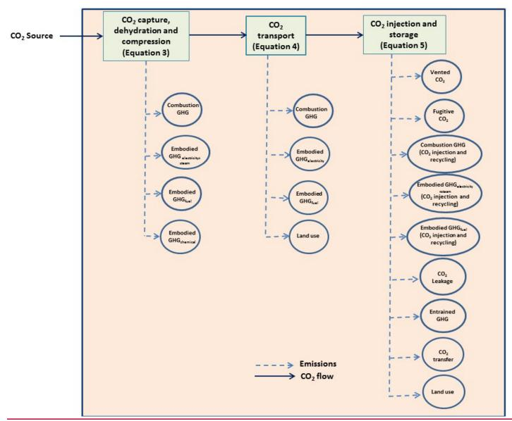
Figure 1. System boundary for CO<sub>2</sub> capture and sequestration in oil and gas reservoirs used for CO<sub>2</sub>-EOR.
