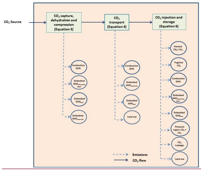
Figure 2. System boundary for CO<sub>2</sub> capture and sequestration in depleted oil and gas reservoirs and saline formations.
