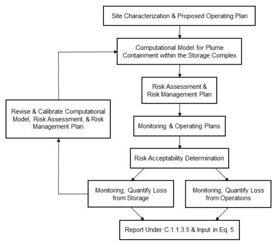
**Figure 4.** Flow chart of showing the process monitoring and modeling for a CCS project design.
