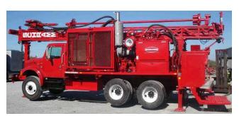
**Two Engine Drill Rig**
