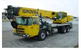
**Two Engine Truck Mounted Crane**
