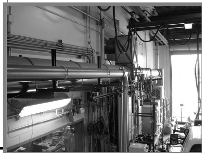
Horiba full flow dilution tunnel
