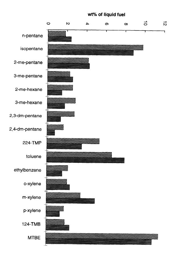
Figure 5: Comparison of Gasoline Composition, Profile 419 (left bars) vs. Bay Area Summer 1996 Composite (right bars)
