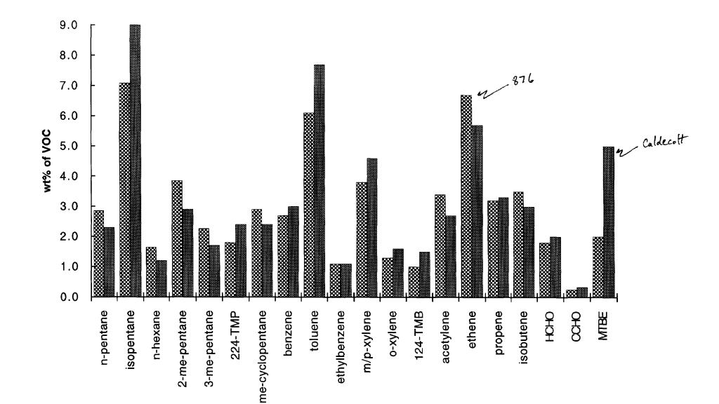
Figure 1: Comparison of Stabilized Exhaust Profile 876 with On-Road Emissions Profile (1996 Caldecott tunnel)
