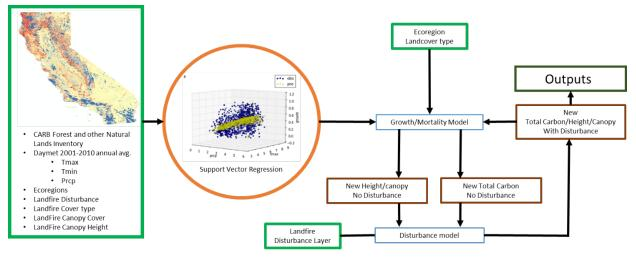
Input datasets are delineated in green boxes. The machine learning algorithm used to derive growth models is in the orange circle. Derived datasets, both internal-interim and outputs, are in brown boxes. Blue boxes represent computations performed.
