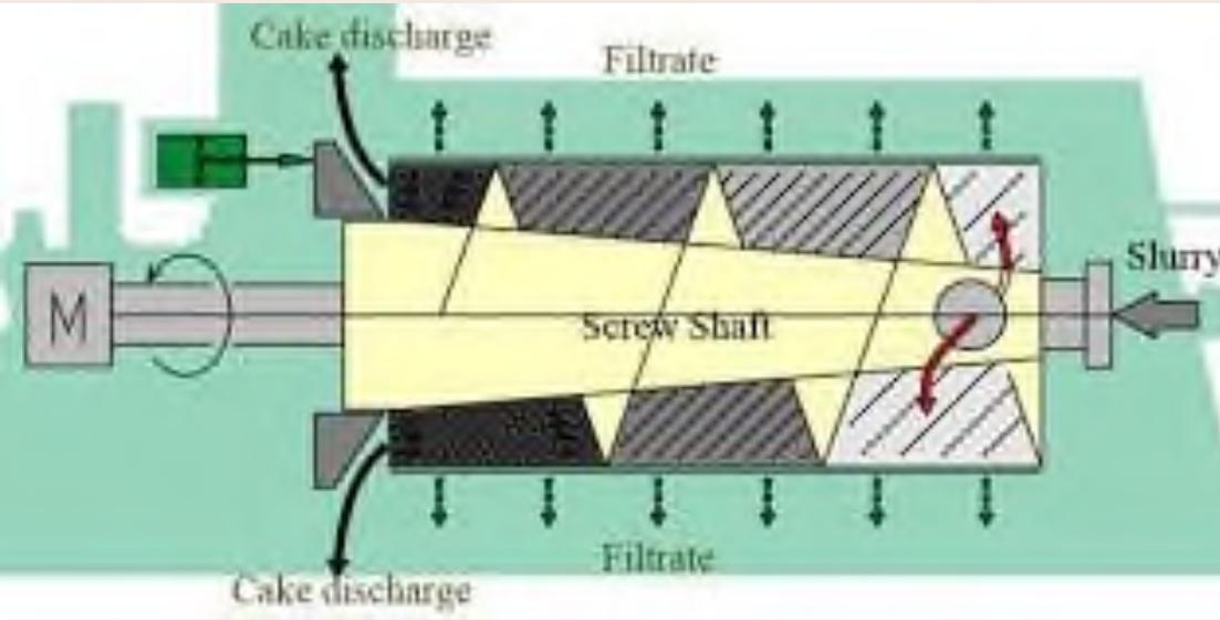
Turns slurry into a stackable product by exerting pressure and squeezing liquid through screen
