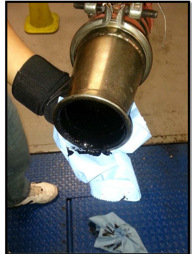
Contamination of CARB emissions lab sample train
