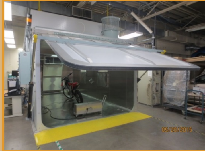
Sealed Housing for Evaporative Determination (SHED)
