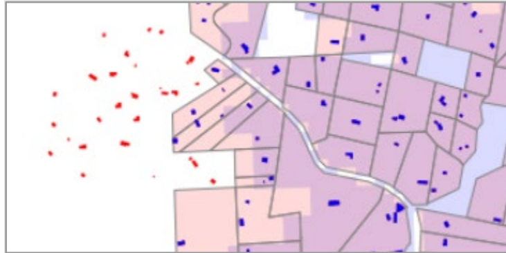
Figure 41: Parcel and structure cleaning. Parcels (pink with grey outline) included in the analysis because they intersect WUI zones (blue shading) and contain at least one structure. Red are structures which were excluded because they do not intersect a WUI zone.
